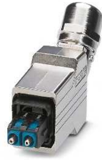
SC-RJ connector, cable outlet at the top, for polymer fibers 980 / 1000 µm
